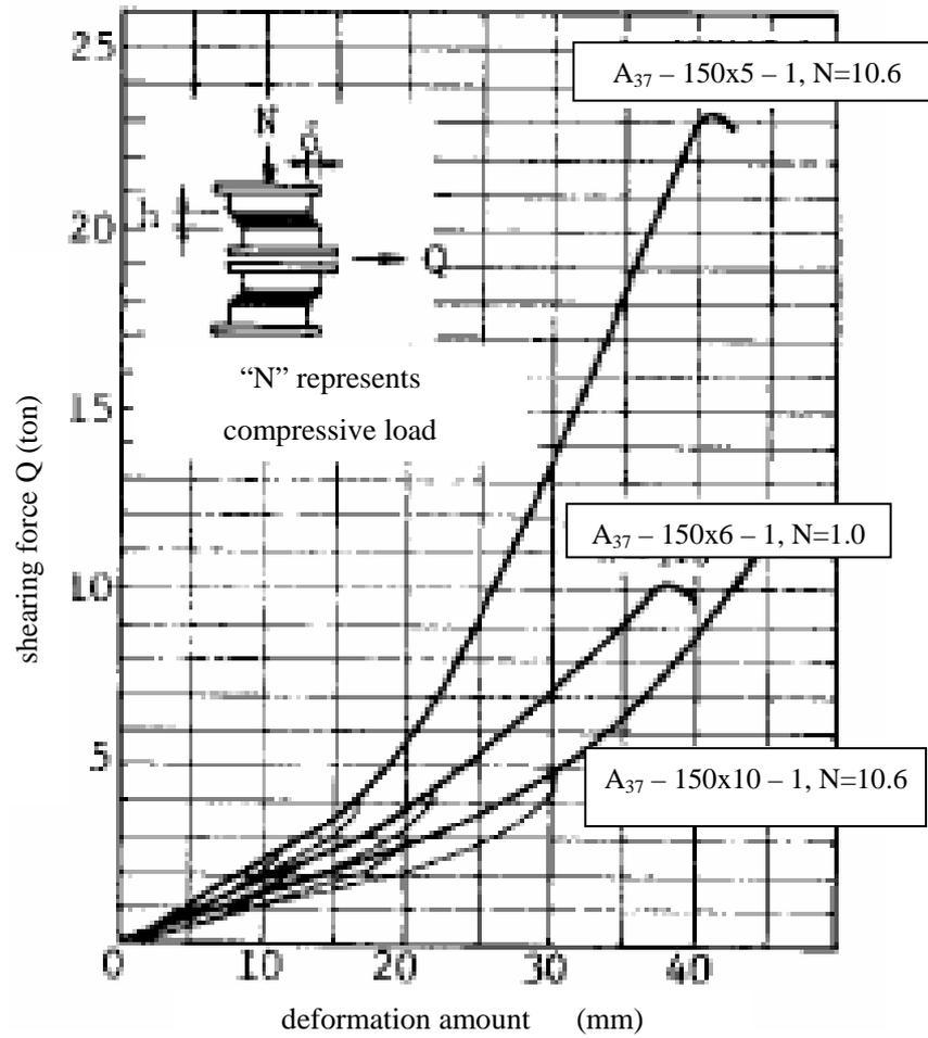
Fig. 3 destruction experiment on single-layer aseismic isolator
