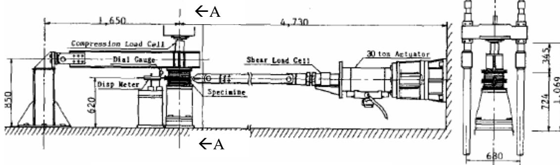
Fig.1 Two-way loading test machine
