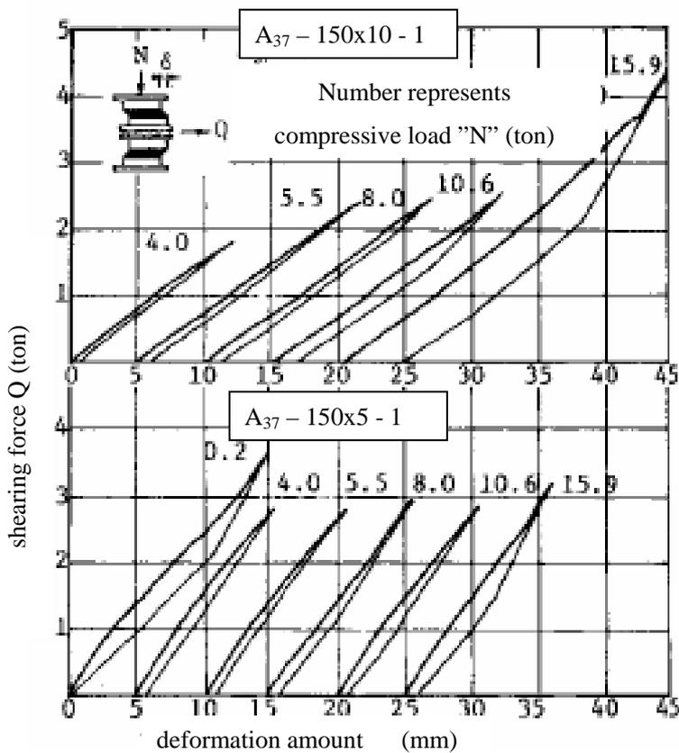
Fig.2 Compressive shearing experiment
